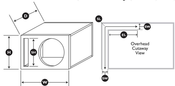
• The enclosure recommendations listed are **external** dimensions which assume the use of **3/4" (19mm)** thick material. If you are using **5/8" (16mm)** thick material, subtract **1/4" (6.5mm)** from each dimension. Do not use any material with a thickness of less than **5/8" (16mm)** as this may compromise the rigidity of the enclosure.
