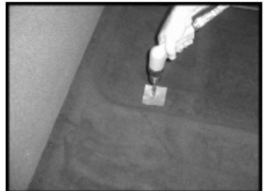
**STEP 10:** Place the Stealthbox into its mounting location, tucking the excess wire neatly out of sight. Turn on the system and test the enclosure's operation before bolting it down.
